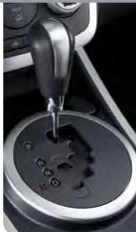
The transmission will automatically adjust how and when it shifts gears based on road conditions and your driving style. The transmission may stay in a lower gear longer than usual when going up or down hills or driving around corners. This feature gives you better control and a more connected driving experience.
